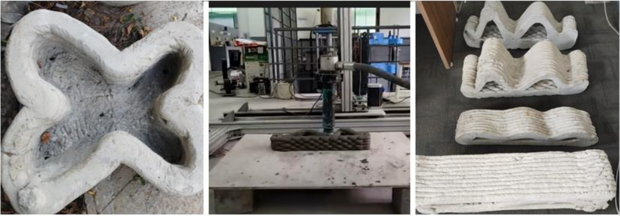
Figure 1 3D Printer and 3D printed Concrete elements
